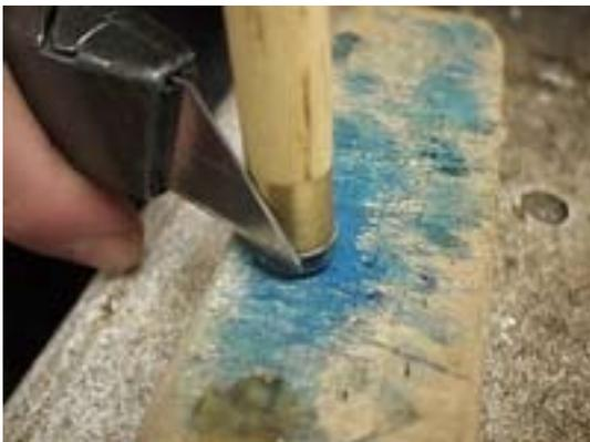
*PHOTO: Carefully cut away the overhanging tip making sure you keep the blade as vertical as possible thereby 'sliding' down the ferrule, using it as a guide, and cutting the tip flush and level. Don't cut or scratch the ferrule.*
