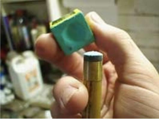
*PHOTO: This is the sort of shape your new tip should have. Not too rounded and not too flat, just a nice gentle dome.*
