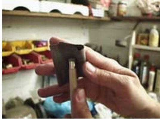
*PHOTO: Be careful to angle the sandpaper away from the cue so that on your downward strokes you don't scratch the ferrule and, more importantly, you don't scratch the shaft of the cue.*
