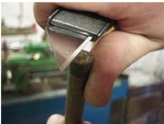
*PHOTO: REMEMBER - You are not trying to make the surface flat with the blade because it should already be flat. You are just trying to remove anything still stuck to the surface.*
