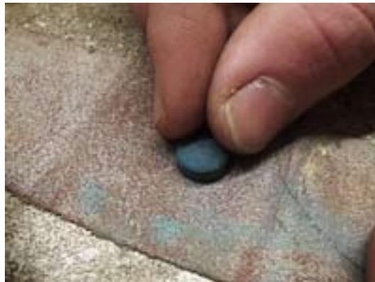
*PHOTO: Try to keep the tip flat as you sand it. If you 'rock' it you will make the surface convex or angles and cause problems when glueing.*
